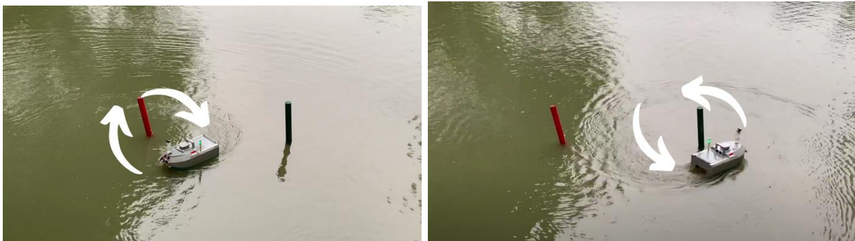
Fig C-5 Maneuver Testing Clockwise and Counterclockwise
